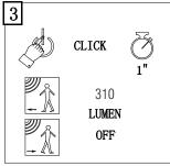
After mode 2, press the switch to change to mode 3. Product will be 310Lm when motion is detected and will turn off after 25 seconds.
