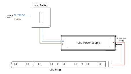
\* Consult switch manufacturer wiring diagram for connections on the switch
