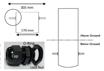
screwing clockwise, when the desired length of cable has been pulled through to reach the bulb holder at the top of the tube with plenty of slack.
