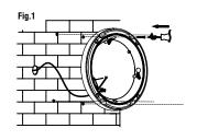
the fixing holes. The casing has 4 "knock outs" for cable or conduit entry. It is necessary to knock out the appropriate panel to allow the supply cable to enter the casing. If using conduit, a hole will also need to be drilled through the outer rim to fit the conduit. The knock out must be fitted with a rubber grommet to protect the cable.
