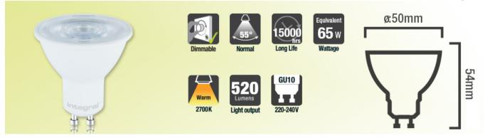
This GU10 lamp offers a wider beam angle of 55 degrees, which will cover a larger area in light with fewer lamps than other GU10 spotlights. The LEDs are specially arranged for a COB-like effect, which paired with the diffuser lens creates a light quality very similar to traditional halogen spotlights.
